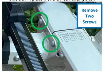
Set the light in place and line up the holes with the screw locations. Insert the new longer screws through the light bracket and thread into the rack holes. Tighten the screws per the rack manufacturers specification.
