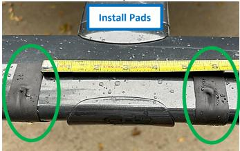
2. Feed the clamps through the bracket mount holes lining up the buckles below the rack. Set the light in place lining it up on the pads.
