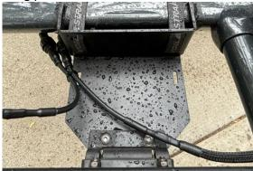
Route cable along rack and test the light.
