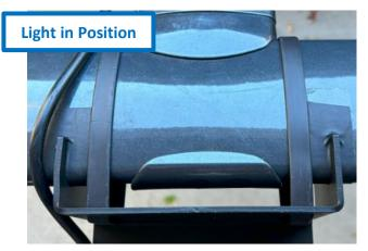
3. Run the Hose Clamps around the bike tray and secure. For the hose clamps, feed the flat end of the clamp into the worm drive screw and tighten the screw until the light bracket is held in place.
