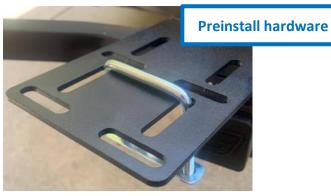
2. Place the light on the rack and position the bracket and U-bolts. Hold the light in place and install the second u-bolt behind the bike tray. Tighten the lock nuts. While loose, the parts will squirm around but as they tighten you can set final position. Don't over tighten as too much torque can bend the bracket.
