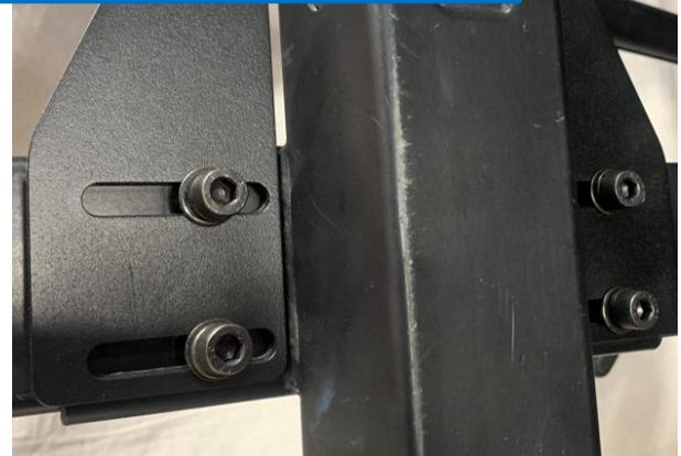
Adjust Tray and Tighten Screws
